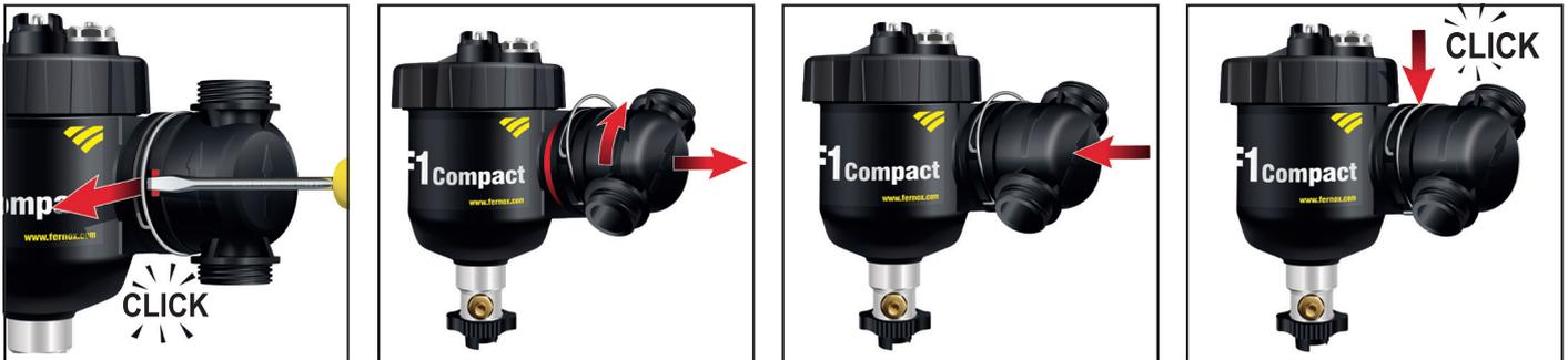
Using a flat end screwdriver in the recess shown, gently lever the locking clip into the 'unlock' position.
