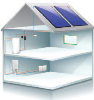
Zenith Solar system Mynute i sealed system boiler Aquaflow Twin coil cylinder
