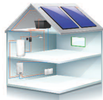
Zenith Solar system Mynute VHE regular open vent boiler Aquaflow Twin coil cylinder
