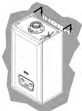
Fig.30 Mounting the boiler
