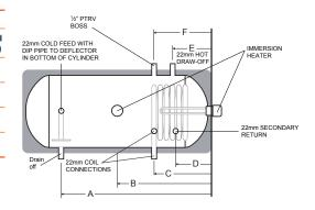
\*Note: 180L & 210L Cylinders fitted with 1 3/4" BSP boss for an additional immersion heater, sold separately. Immersion heater CODE: IMHTRSS All dimensions are in mm
