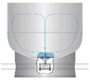
Flow-Thru  $^{\text{™}}$  technology assures total recirculation of the tank's water content.
