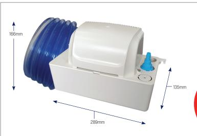
The 5.5 metre discharge lift helps with the flexibility of the installation. Suitable for both floor and wall mounting and comes with a quick release check valve. Suitable for boilers up to 200kW this version comes with 6 metres of 9.5mm (3/8") ID flexible drain hose.
