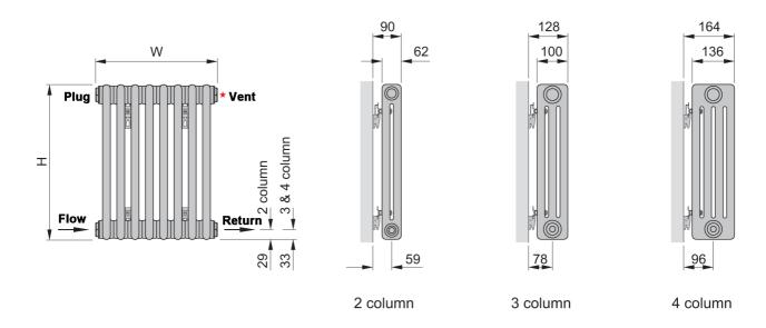
Please note that due to the unique flow diverter built within all Revive column radiators the flow needs to be on the same side as the permanent blank which is the opposite side to the air vent bleed valve. (As indicated above)
