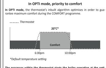
The processor within the thermostat starts the boiler operation at the optimum time to achieve the setpoint temperature at the start of the occupancy period.
