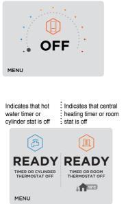
Indicates that boiler Boiler is providing is heating the hot central heating and water cylinder to 60°C radiator temp is 60°C.
