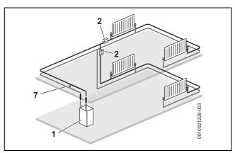
Fig. 7 Separated heating zones
