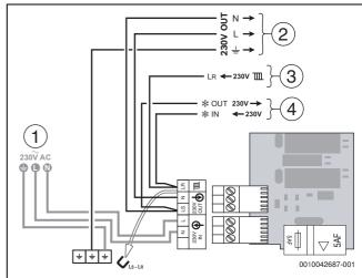
Fig. 60 External controls connections example
