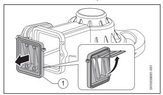
Fig. 77 Non-return valve (bearing plate) in the mixing unit Refer to figure 78.
