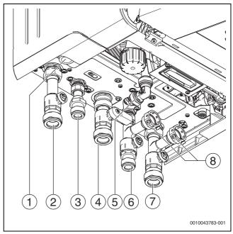
Fig. 44 Connections on the gas and water side
