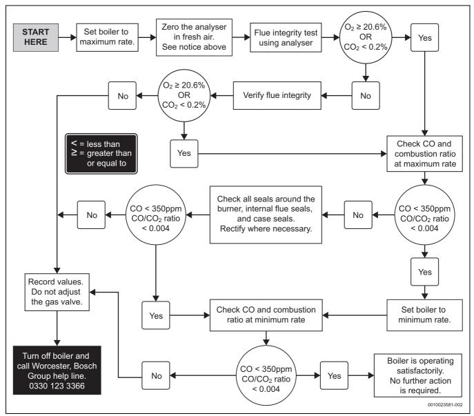
Fig. 68 Commissioning checks flow chart
