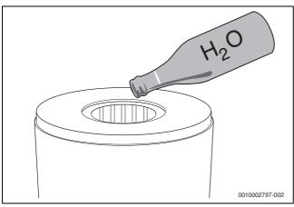
Fig. 81 Rinse the heat exchanger with water
