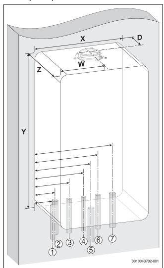
Fig. 2 Pipe and flue outlet dimensions
