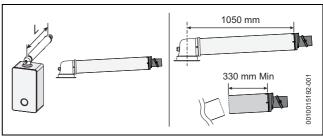
Fig. 16 Horizontal flue option
