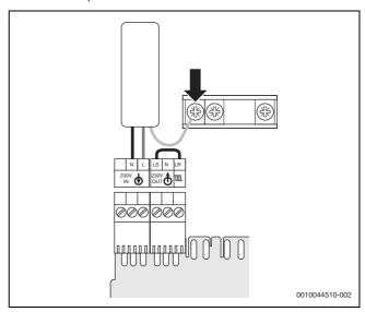
Fig. 56 Connect the power cable
