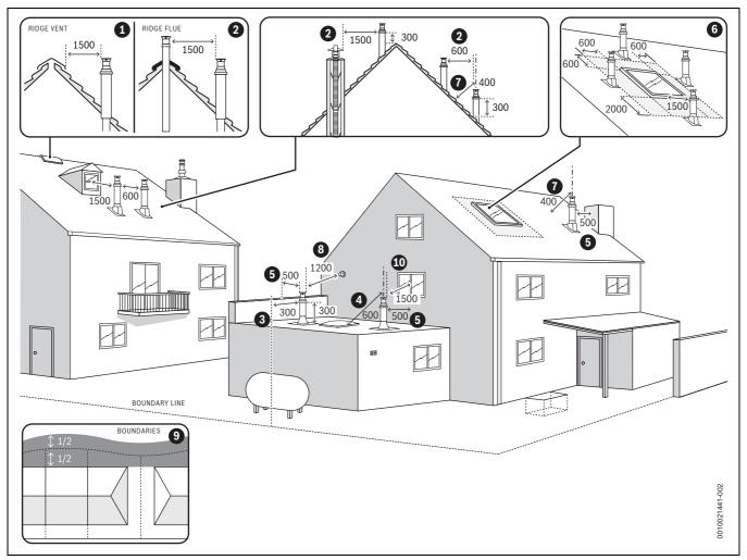
Fig. 28 Vertical flue terminal positions
