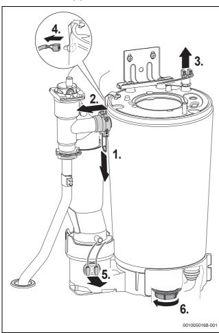
Fig. 109 Separating components from the heat exchanger assembly Removing the heat exchanger assembly Refer to figure 110.
