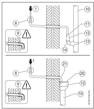
Fig. 35 Disposal into rain water down pipe
