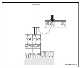
Fig. 57 Connect the power cable
