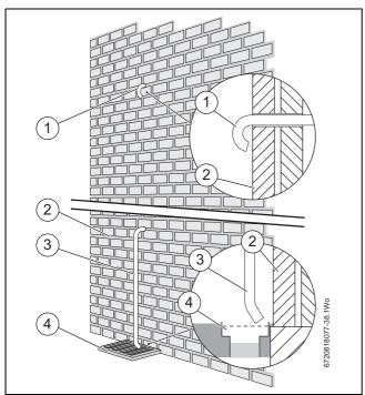
Fig. 39 Pressure relief pipework
