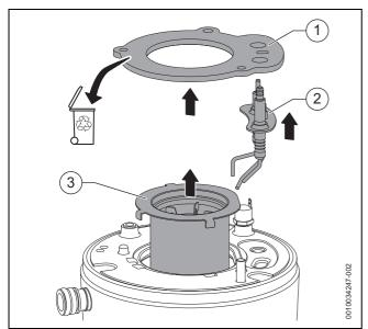
Fig. 78 Removing the burner
