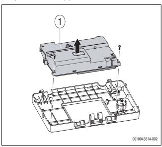
Fig. 111 Replacing the control unit
