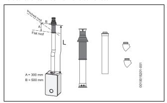
Fig. 25 Vertical flue option
