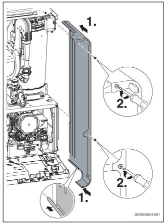
Fig. 113 Attaching the side panel
