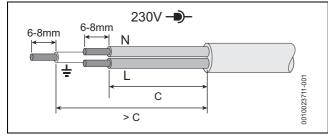
Fig. 58 Mains voltage (power cables) preparation
