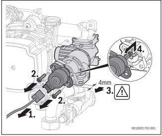
Fig. 107 Detaching the motor from the 3-way valve Installing the motor.
