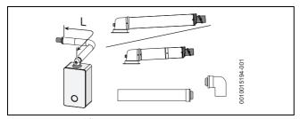
Fig. 18 Horizontal flue option
