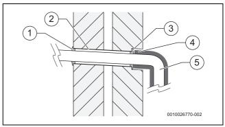
Fig. 34 Additional protection for transition through a wall
