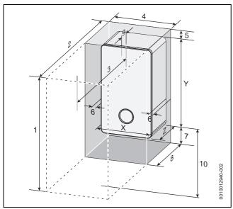
Fig. 11 Appliance minimum clearances
