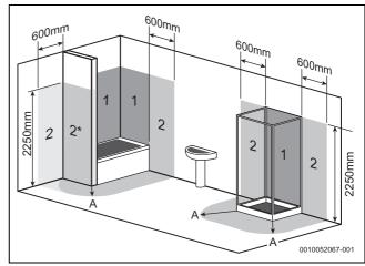
Fig. 10 Bathroom installations
