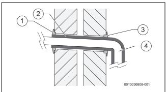
Fig. 38 Through the wall lagging example
