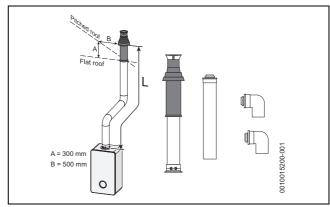
Fig. 24 Vertical flue option
