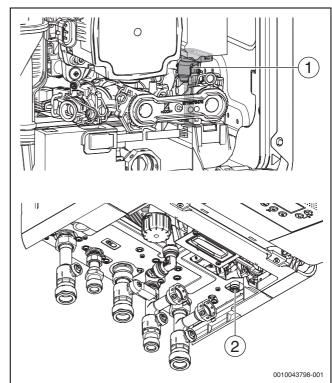
Fig. 90 Drain point
