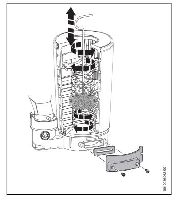
Fig. 80 Cleaning the heat exchanger
