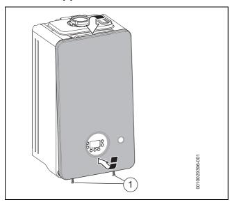
Fig. 71 Fitting the front panel
