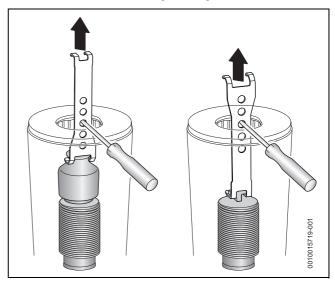
Fig. 79 Remove the top and bottom baffles
