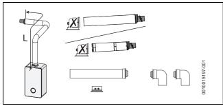
Fig. 21 Horizontal flue option
