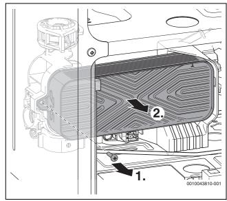
Fig. 102 Removing the plate heat exchanger
