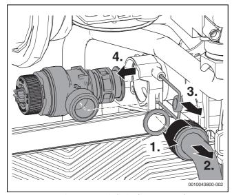
Fig. 91 Remove the pressure relief valve (heating circuit)
