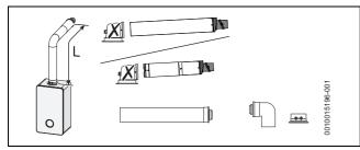
Fig. 20 Horizontal flue option
