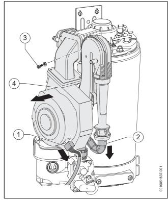
Fig. 75 Removing the fan with mixing unit
