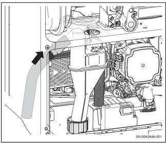
Fig. 46 Fitting the hose to the condensate trap
