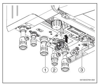
Fig. 43 Connecting to the PRV tail connection
