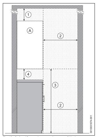
Fig. 12 Reduced front maintenance clearances - Side view
