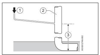
Fig. 31 Disposal to soil vent stack
