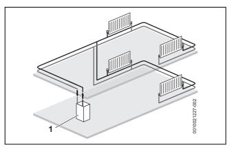
Fig. 6 Single central heating circuit example
