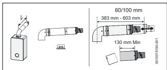
Fig. 14 Horizontal flue option
