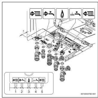
Fig. 42 Fitting the connection sets (for orientation reference)
