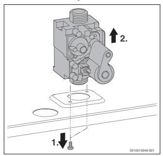
Fig. 104 Removing the gas valve
