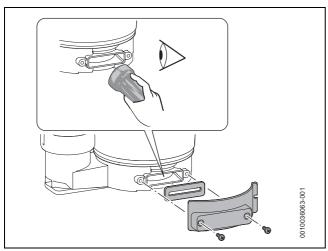
Fig. 82 Checking the heat exchanger for residue
