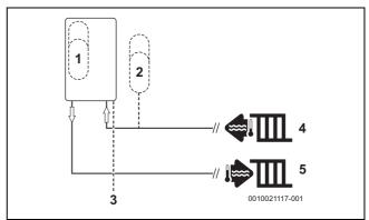
Fig. 4 Additional expansion vessel
