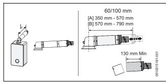
Fig. 15 Horizontal flue option
