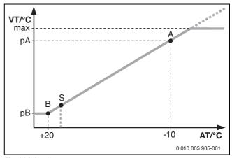
Fig. 116 Heating curve
