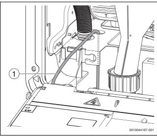
Fig. 51 Mains supply cable routing
