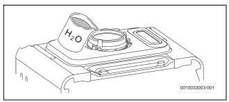
Fig. 47 Filling the siphon
