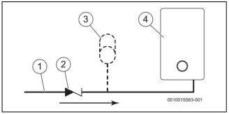
Fig. 9 Mini expansion vessel location
