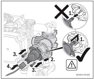
Fig. 108 Installing the motor in the 3-way valve
