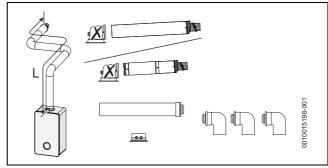
Fig. 22 Horizontal flue option
