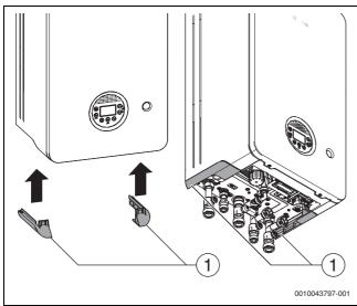
Fig. 72 Assembly direction of infills
