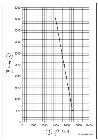
Fig. 27 Plume length to flue length graph
