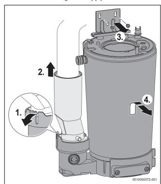
Fig. 110 Removing the heat exchanger assembly
