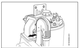
Fig. 74 Test nipple at the mixing device
