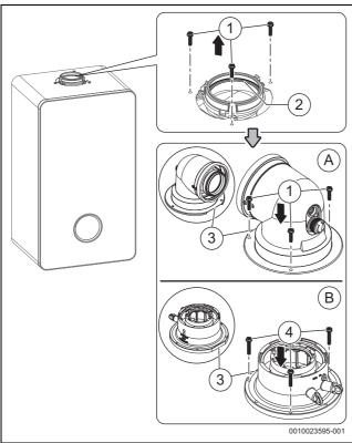
Fig. 49 Flue turret/adaptor connection
