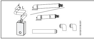
Fig. 19 Horizontal flue option
