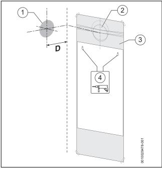
Fig. 41 Wall mounting template
