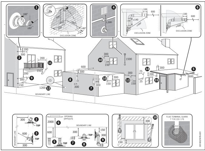
Fig. 30 Plume re-direct and plume management terminal positions
