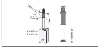
Fig. 23 Vertical flue option
