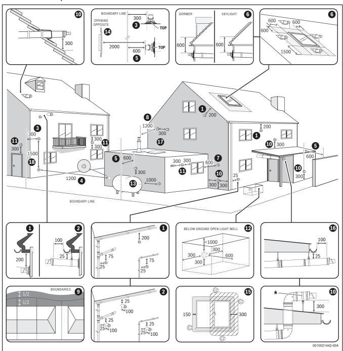
Fig. 29 Horizontal flue terminal positions
