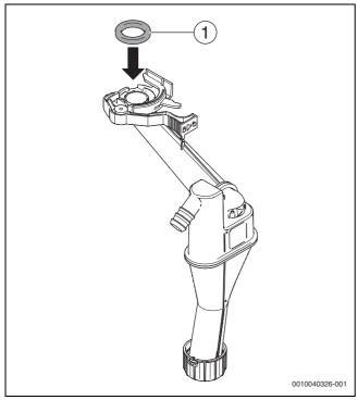
Fig. 85 Inserting the gasket on the condensate trap
