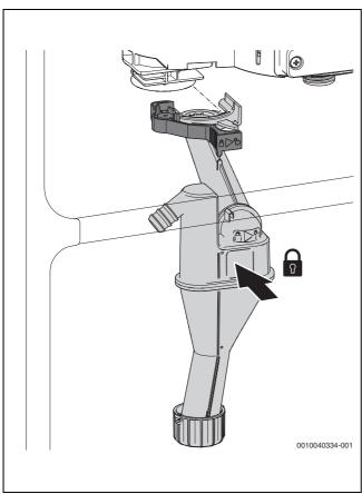
Fig. 86 Inserting the condensate trap
