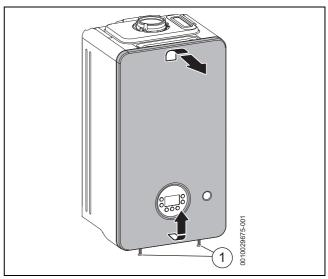
Fig. 40 Removing the front casing
