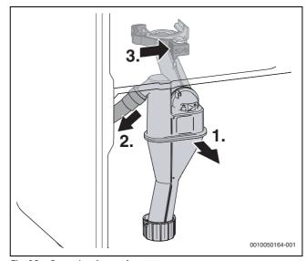
Fig. 83 Removing the condensate trap
