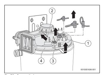
Fig. 76 Remove the burner cover
