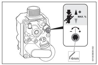
Fig. 88 Setting the CO<sub>2</sub> content
