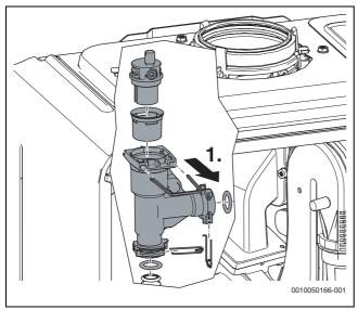
Fig. 106 Removing the automatic air vent valve
