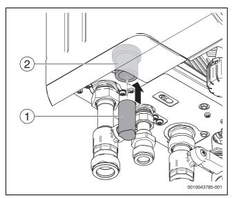
Fig. 45 Connecting to the condensate outlet connection
