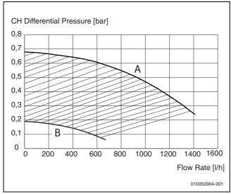
Fig. 61 Circulation pump characteristic curve
