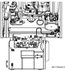
Fig.41 Connecting the room thermostat RT
