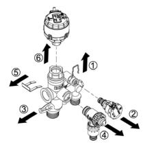
Fig.78 Removing the pump
