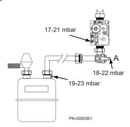
Fig.47 Gas inlet test point
