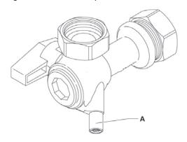
Fig.48 Type of fittings — flue gas measuring point
