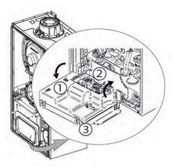
Fig.39 Adding wires to the PCB
