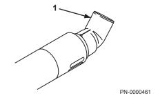
Push the flue deflector over the terminal end. It may point upwards as shown, or up to  $45^\circ$  either way from vertical. Secure the deflector to the terminal with screws provided.
