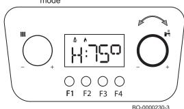
3. Turn the knob another notch to the right. When the letter **H** appears on the display (followed by the flow temperature) the boiler is working at maximum power in DOMESTIC WATER MODE.
