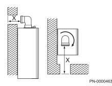
Fig.36 Flue dimension Y
