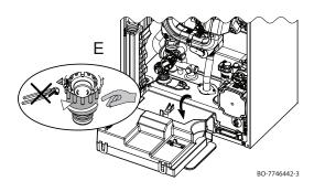
The drain cock is inside the boiler (in the lower left-hand section). To access the cock and drain it, proceed as follows:
