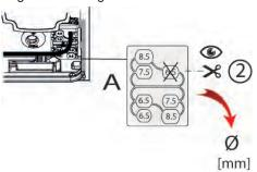
Fig.40 Connecting wires to the PCB
